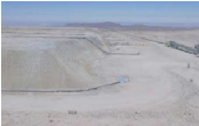
Photo 1 : Biolixiviation en tas (Mine Cerro Colorado Chile, 100 000 t/an)
